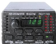
Digital 24-Bit Multifunction Signal Processor
